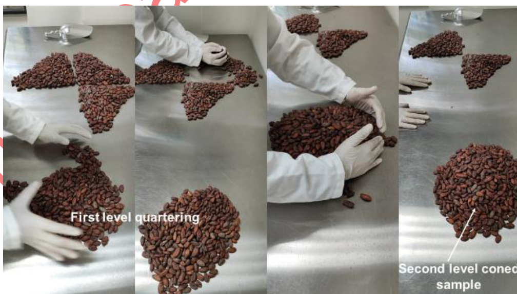
Figure E. 2: Reducing the composite sample
