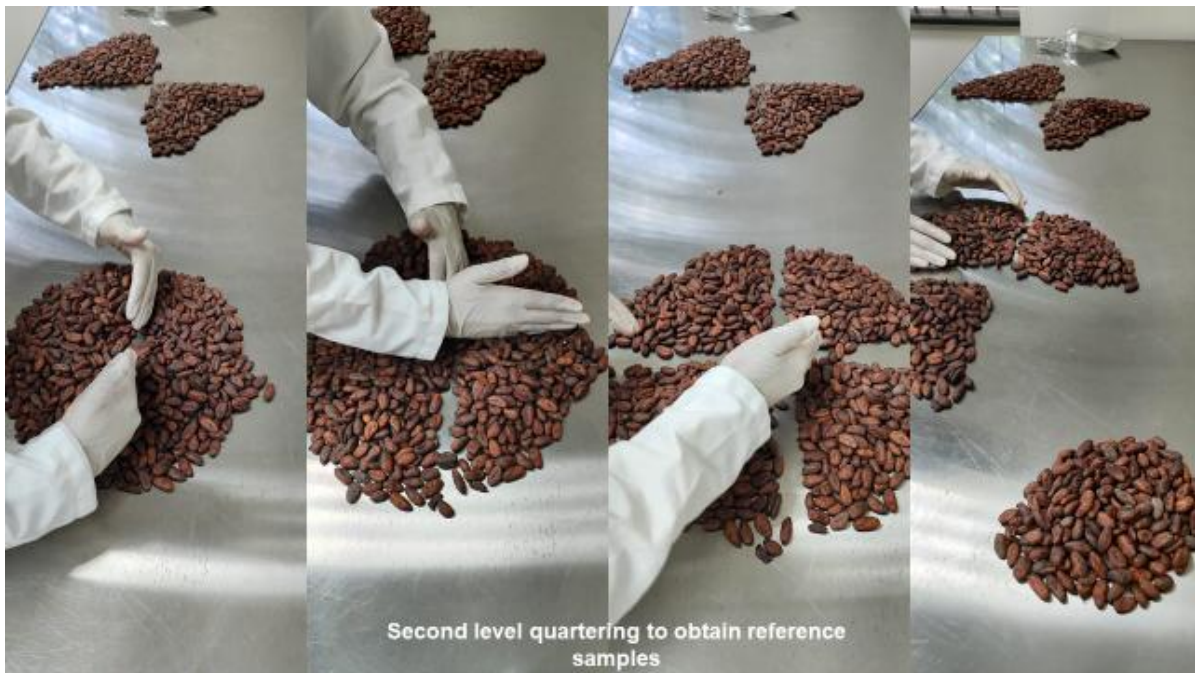
Figure E.3: Coning and quartering to obtain reference samples
