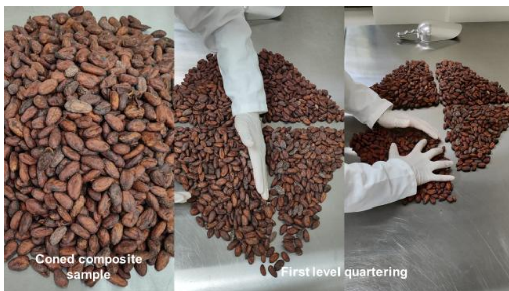
Figure E. 1: Coning and quartering of composite sample
