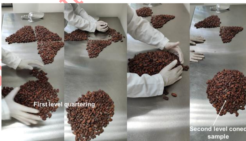
Figure E. 2: Reducing the composite sample
