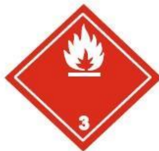
Figure 2 — Sample pictogram for the labelling of a flammable liquid for transport, in the UN Model Regulations. (Symbol: Flame: black or white Background red; Figure 3 in bottom corner; minimum dimensions 100 mm x 100 mm)
